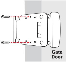
1. Attach latch to side of gate with two screws
