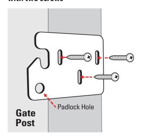
4. Place strike plate on gate post and align padlock holes with latch. Install three screws. Slots allow vertical adjustment.
