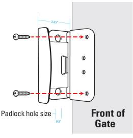
2. Secure latch to front of gate with two screws
